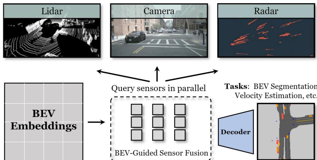
**Input:** Sensory measurements (RGB, Lidar Points, Radar Points, etc.)
