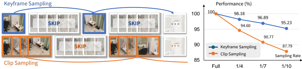
Figure 7: Evaluation on different video downsampling strategies for V-JEPA on the segmentation task. Keyframe Sampling samples every N frames to form a new video sequence, while Clip Sampling directly samples consecutive video clips. The performance before downsampling is regarded as 100%. Keyframe sampling demonstrates less performance drop with the same level of downsampling.
